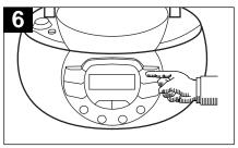
Press either the Skip/Search Repeat step 5 until you have FWD. (►►) or REV. (◄◄) button programmed up to 20 track • to select the next track you numbers into the CD Program Memory. After programming up to wish to program (Example: Track 20 tracks in the CD Program 8). When Track 8 appears in the display, press the CLOCK Memory, press the CD PLAY/PAUSE (►III) button to begin programmed playback. "MEMORY" will appear in the display and playback will begin on the first track that you programmed.
